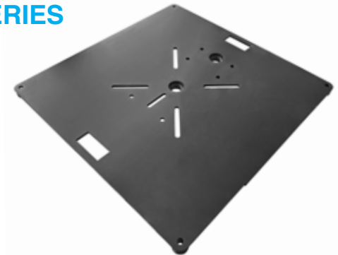
BP3636-STEEL-TS-2F STEEL 36" x 36", 9mm thick top plate with 2 welded 1-1/2" schedule 40 flanges
