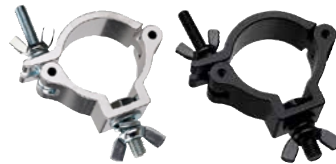
Medium-Duty Coupler with Standard Wing Nut, Fits 1.9-2" OD Tube, 165 lb Load
