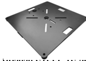
BP3030-STEEL-1S-2F STEEL 30" x 30", 9mm thick top plate with 2 welded 1-1/2" schedule 40 flanges
