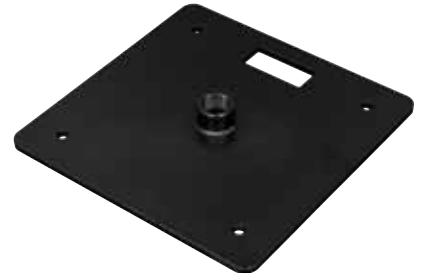
BP1919-STEEL-FLAT-1F STEEL 19" x 19", 12mm thick 50 lbs. base plate with welded protruded 1-1/2" schedule 40 flange
