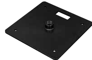
BP1919-STEEL-FLAT-1F STEEL 19" x 19", 12mm thick 50 lbs. base plate with welded protruded 1-1/2" schedule 40 flange
